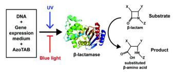
Using a custom-built photosensitive nucleic acid binder, a commercially available gene expression system, and  $\beta$ -lactams as target enzyme substrates, the authors show that a short UV illumination triggers  $\beta$ -lactamase synthesis and the subsequent
